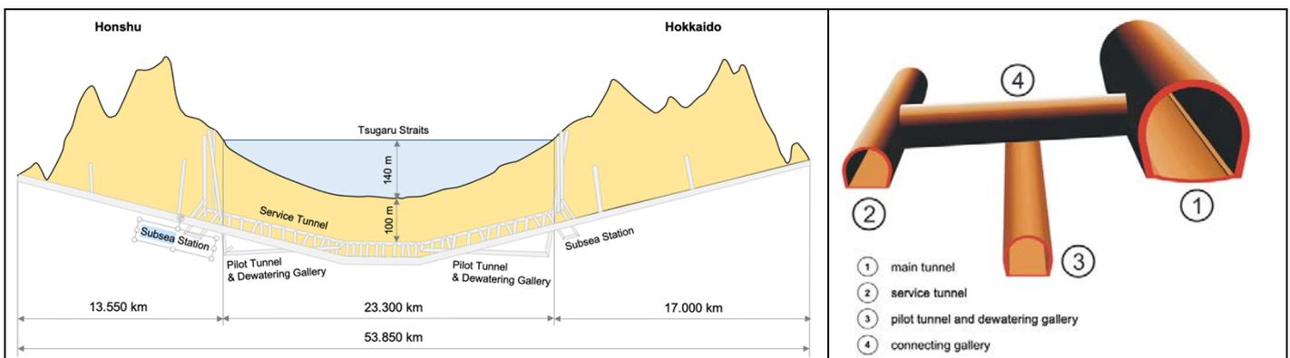
Figure 3. Tunnel System of the Seikan Tunnel (source: Wikipedia)
