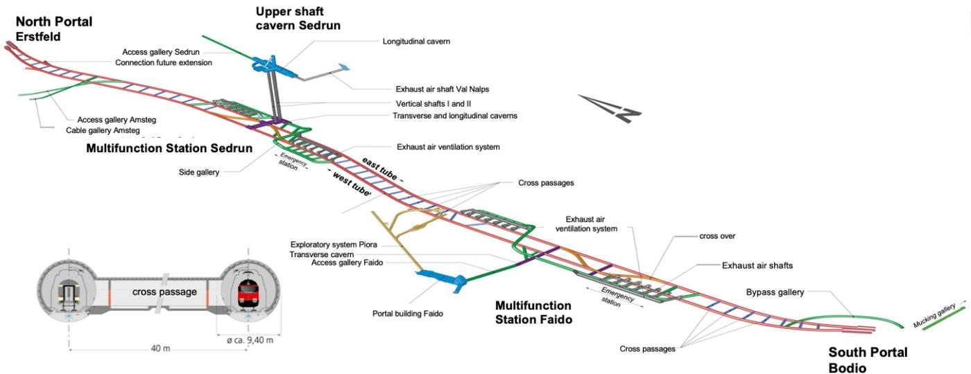
Figure 5. Tunnel System Gotthard Base Tunnel (Source: Amberg Engineering, STS 2016)
