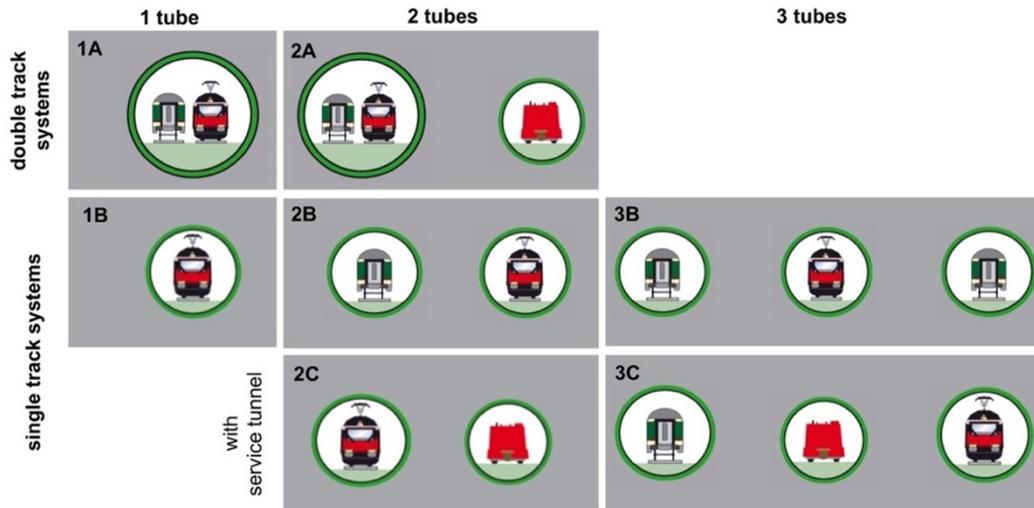
Figure 2. Variants of railway tunnel systems
