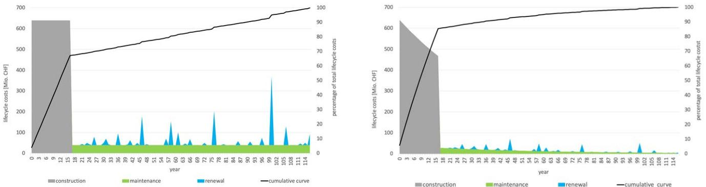
Figure 11: Life cycle cost (17 years construction time, 100 years of operation) without interests and inflation (left) and with 3% interests, 1% inflation (right) (Tannó, 2018)
