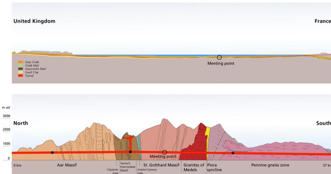
Figure 1: Longitudinal profile of a subsea tunnel (Eurotunnel) and a mountain base tunnel (Gotthard Base Tunnel) (source Wikipedia and AlpTransit Gotthard)
