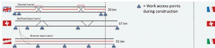
Figure 7. Systems layout of long tunnels in Europe with work access points during construction (FINEST LINK, 2018).
