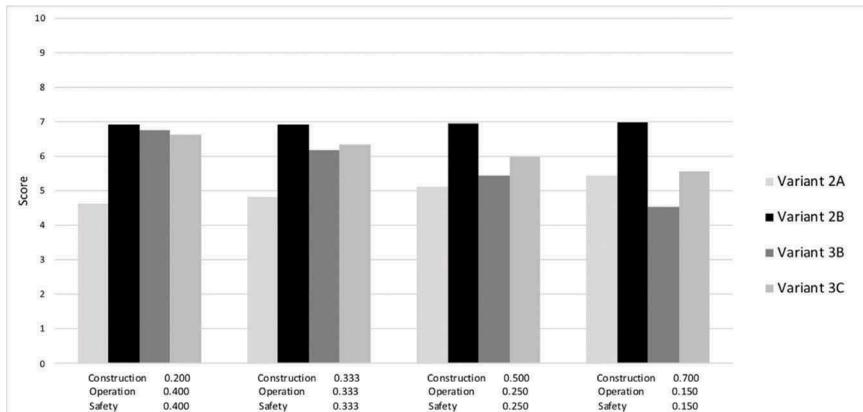
Figure 5. Scores in value-benefit analysis for the Swiss NRLA-base-tunnels (based on EBP, 1993).
