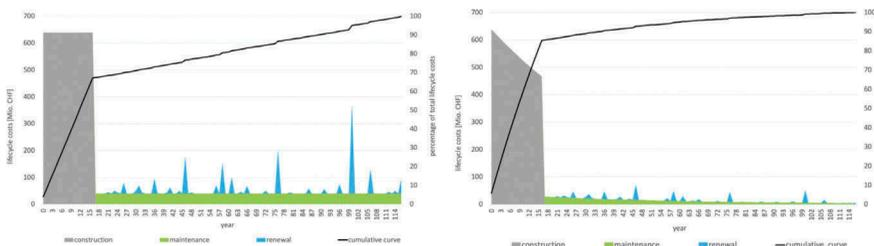
Figure 8. Life cycle cost (17 years construction time, 100 years of operation) without interests and inflation (left) and with (3% interests, 1% inflation right) (Tannò, 2018).
