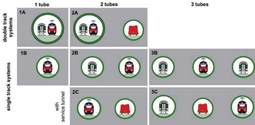
Figure 1. Variants of railway tunnel systems.
