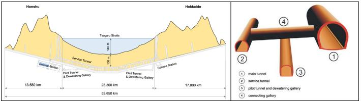
Figure 3. Tunnel System of the Seikan Tunnel (source: Wikipedia)
