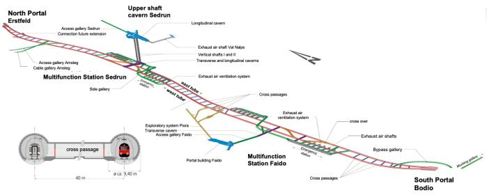
Figure 5. Tunnel System Gotthard Base Tunnel (Source: Amberg Engineering, STS 2016)
