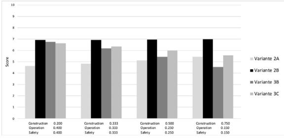
Figure 9: Scores in value-benefit analysis for the Swiss NRLA-base-tunnels (based on EBP, 1993)
