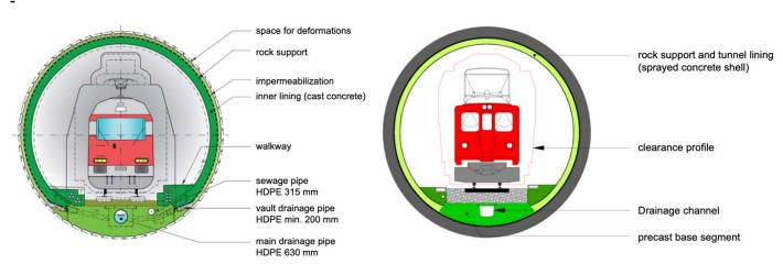
Figure 6. Typical Tunnel cross sections for the double lined Gotthard Base Tunnel (left) and the single lined Vereina Tunnel (right) (Source: Amberg Engineering)
