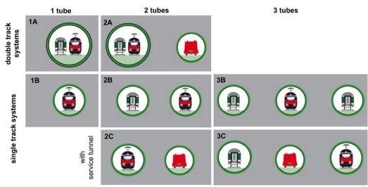
Figure 2. Variants of railway tunnel systems
