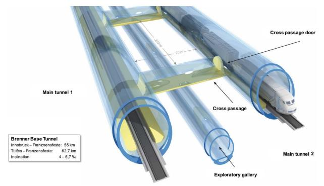
Figure 13: Tunnel System for the Brenner Base Tunnel (source BBT SE)
