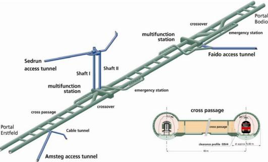
Fig. 3: Scheme of tunnel system, Gotthard Base Tunnel
