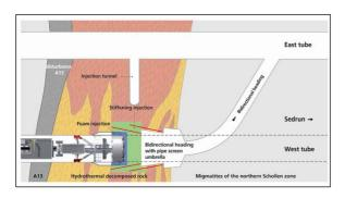
Figure 15: Overcoming a fault zone at Amsteg
