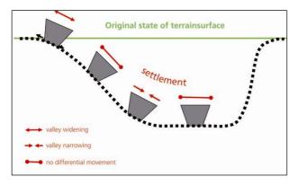
Figure 9: Effects of surface deformations on structures
