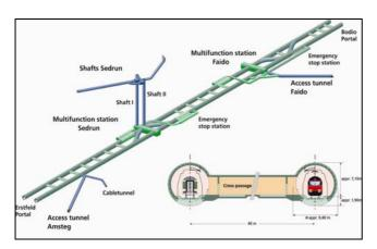
Figure 1: Gotthard Base Tunnel: Overview
