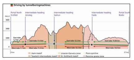
Figure 2: Gotthard Base Tunnel: general longitudinal profile with excavation methods
