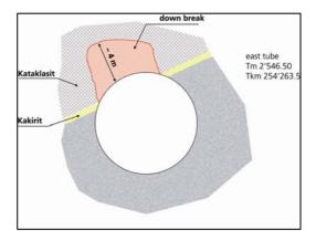
Figure 14: Horizontal fault zone at Bodio
