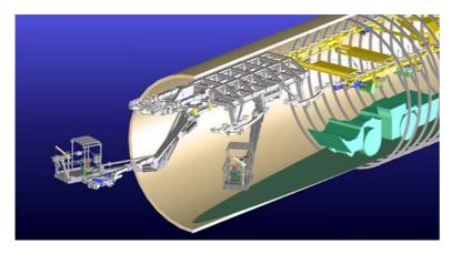
Figure 8: GTA 7500 tunnel lining machine (ROWA)
