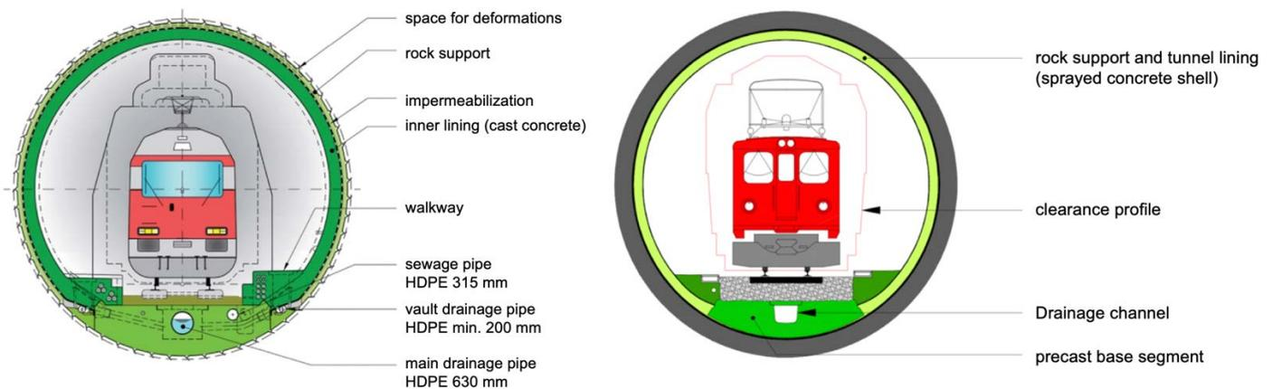
Figure 6. Typical Tunnel cross sections for the double lined Gotthard Base Tunnel (left) and the single lined Vereina Tunnel (right)
