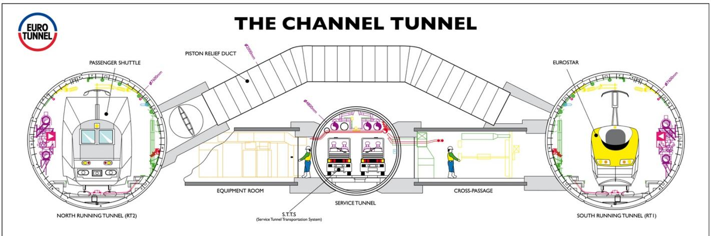
Figure 4. Tunnel System of the Eurotunnel (Source: Eurotunnel)
