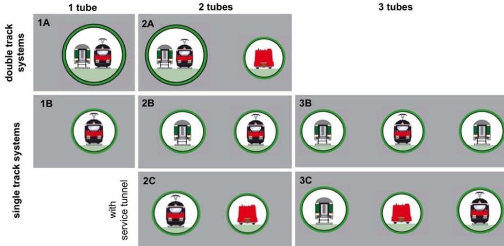
Figure 2. Variants of railway tunnel systems
