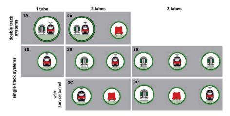
Figure 1. Variants of railway tunnel systems.
